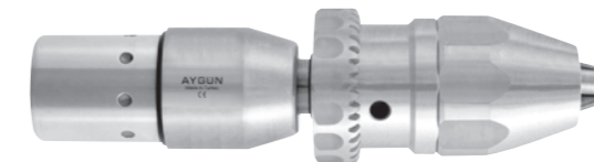
M208-310 Drill attachment with hybrid chuck Both keyed and keyless operation Ø4 mm Cannulated Ø 1.0 mm - 7.4 mm 900 rpm / 4 Nm 34 x 142 mm / 485 g
