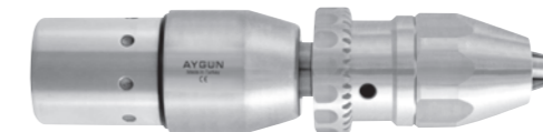
M208-313 Drill attachment with hybrid chuck Both keyed and keyless operation Ø4 mm Cannulated Ø 0.3 mm - 3 mm 900 rpm / 4 Nm 30 x 130 mm / 395 g
