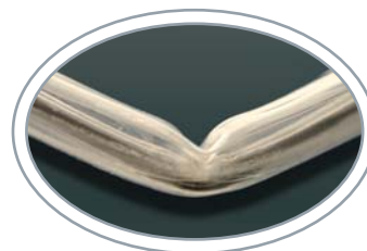
Polyurethane catheter Sample of competitor's polyurethane catheter at a 20% bend.
